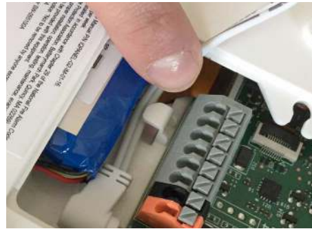
Route the wire behind the retainer clip
