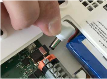
Plug in the power connector
