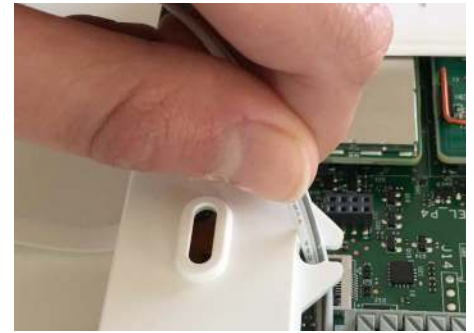
Insert the wire into the strain-relief
