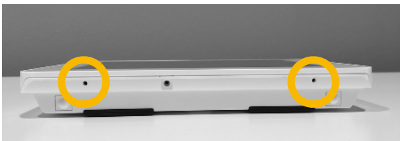
Microphones are located on the bottom of the panel
